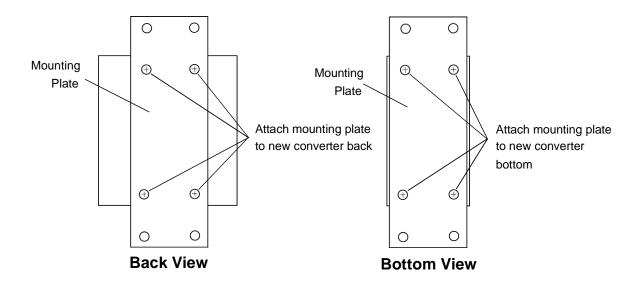
4. Secure the converter to the mounting surface with four screws through the holes in the mounting plate.
